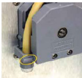
Figure 10-7: Inserting New Tubing
