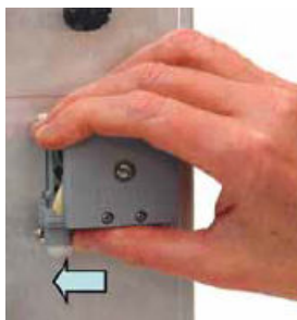
Figure 10-6: Pushing the Tubing Fitting Out
